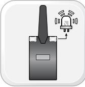
The antenna's LEDs will flash once [1x] for each successful pairing.
