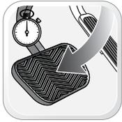
Press and hold the brake pedal.
