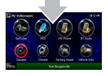
Maestro features can be accessed in the My Volkswagen submenu. If an icon is not active (grayed out) then it is not available in your vehicle or it was disabled when the Maestro module was programmed using Weblink. The options described here may not be available in your vehicle.
