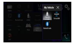
Press on Satellite Radio to listen to the factory satellite radio tuner. This allows you to use the tuner that's already in your vehicle, rather than installing an aftermarket tuner. Your vehicle must be equipped with a tuner for it be retained by the Maestro RR module.
