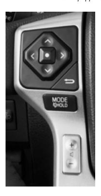
Your steering wheel buttons can be used to control your aftermarket Pioneer radio. You can assign steering wheel buttons to Pioneer radio functions. Simply program your Maestro RR module online using the Weblink updater and customize your buttons. Each steering wheel button can control up to two radio features.
