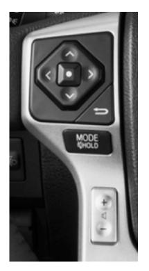
Your steering wheel buttons can be used to control your aftermarket Pioneer radio. You can assign steering wheel buttons to Pioneer radio functions. Simply program your Maestro RR module online using the Weblink updater and customize your buttons. Each steering wheel button can control up to two radio features.
