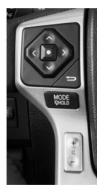
Your steering wheel buttons can be used to control your aftermarket Kenwood radio. You can assign steering wheel buttons to Kenwood radio functions. Simply program your Maestro RR module online using the Weblink updater and customize your buttons. Each steering wheel button can control up to two radio features.
