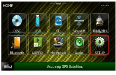
When parking assist interrupt is set to ON, the Maestro parking assist screen will pop up when the vehicle is in reverse. If the vehicle is also equipped with a backup camera, there is also a reverse interrupt setting for it in the radio. Only one feature's reverse interrupt should be set to ON, or there will be a conflict in the radio.
