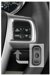
Your steering wheel buttons can be used to control your aftermarket Pioneer radio. You can assign steering wheel buttons to Pioneer radio functions. Simply program your Maestro Rr module online using the Weblink updater and customize your buttons. Each steering wheel button can control up to two radio features.
