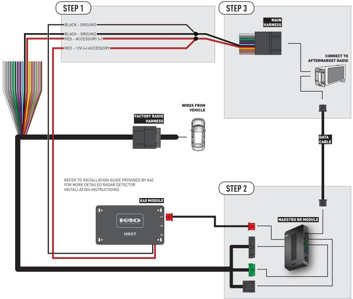
REFER TO VEHICLE SPECIFIC WIRING GUIDE FOR DETAILED RADIO INSTALLATION INSTRUCTIOINS.
